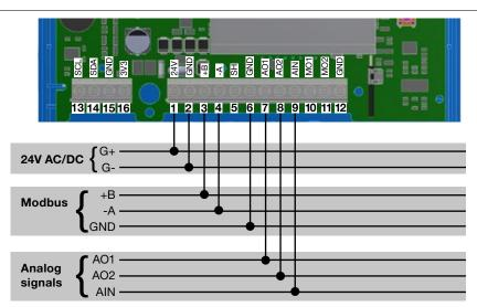
\*) When using AC terminal 1 (G) should have system potential and terminal 2 (G0) should be system neutral.
