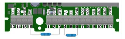
you can add biasing resistors in the screw terminal on <u>one</u> of the UltraLinks to see if this is the cause of the communication failure. Use  $500 - 1000 \Omega$  resistors and connect one resistor from -A to GND and one from +B to the 3V3 terminal. It is also recommended to add a  $120 \Omega$  termination resistor between -A and +B on the last UltraLink on the bus to avoid signal reflections.
