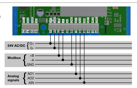
\*) When using AC terminal 1 (G) must have system potential and terminal 2 (G0) must be system neutral.
