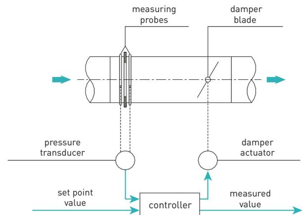
Figure 1. VAV regulator operation.
