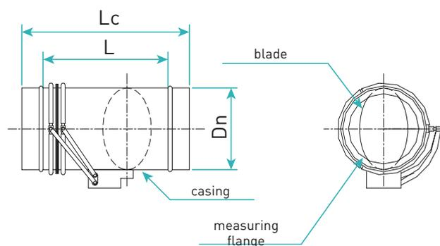
Figure 2. VAV regulator type: RVP-R.
