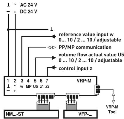
Diagram 3. Connection diagram of the regulator with fast automatic control (VRP-M).
