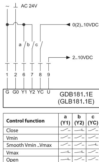
Diagram 2. Diagram of connection between the regulator and the compact cylinder GDB 181.1 or GLB181.1.
