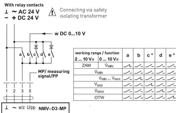
Diagram 1. Diagram of connecting the regulator with a compact actuator NMV-D3-MP or LMV-D3-MP.
