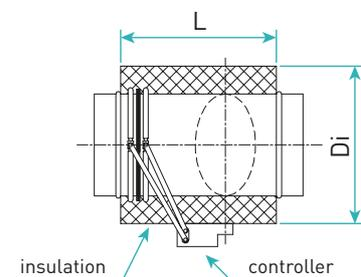
Figure 3. VAV regulator type: RVP-Rt (with insulation).
