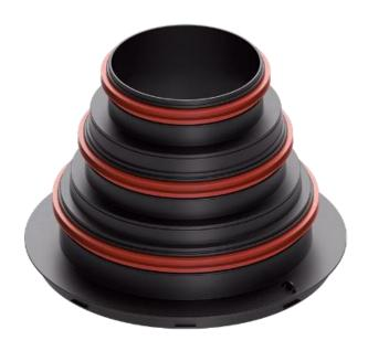
The main central connector is used to connect the main supply air pipe or the main exhaust air pipe to the distribution box. The unused part which diameter is smaller than that of the pipe should be cut off.
