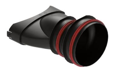
The side connector is used to connect the main supply air or exhaust air pipe to either side of the distribution box. It is designed to be fixed into the oval slot on either side of the distribution box replacing one 3x75 module. If a 125 mm diameter pipe is used, the unused part should be cut off.
