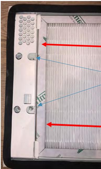
Countersunk M8 nuts holding top clamp. Push towards frame (red arrows) when re-tightening
