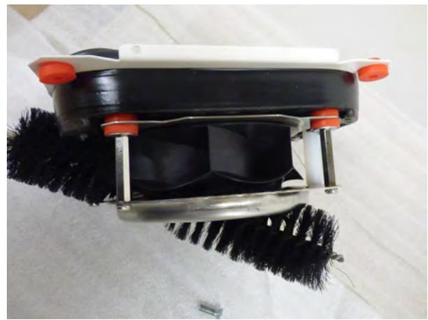
*Figure 163 Brush dirt from impeller*
