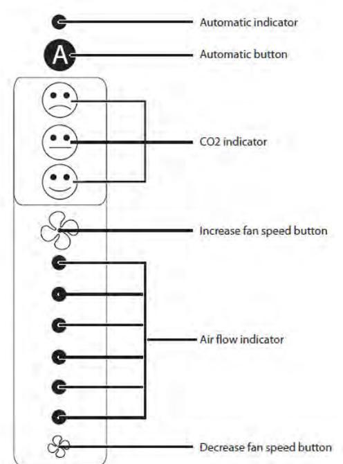
Figure 2 Control panel user interface
