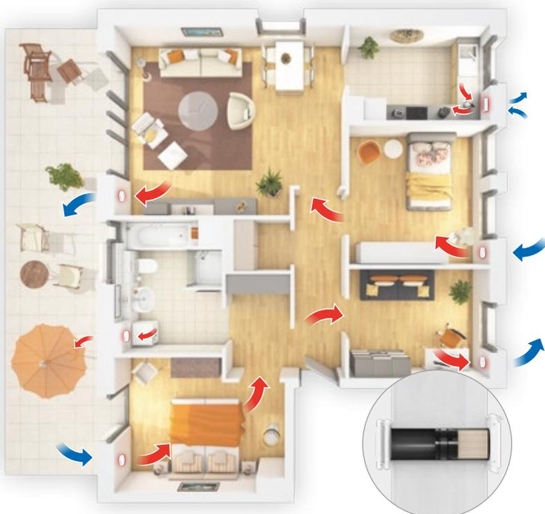
The inVENTer decentralised ventilation system consists of units arranged in pairs. The integrated Xenion® fans bring fresh air to the inside and remove stale air in a coordinated manner. They change their direction of rotation every 70 seconds. The heat is absorbed by the ceramic accumulator and released again. A large part of the heat is retained and you save valuable heating energy.
