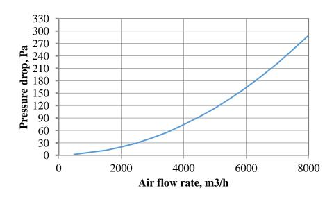
**Diagram of pressure drop loss**: tested filter 592x592x292
