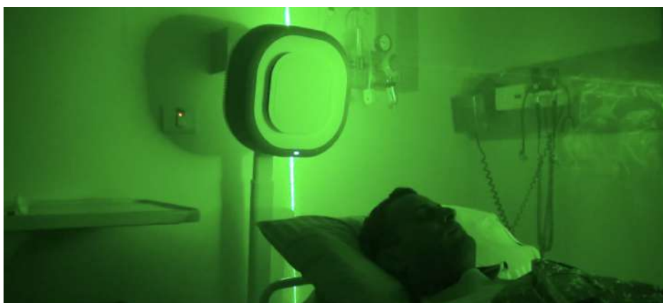
Using a laser light sheet of nearly constant intensity, smoke particles were illuminated in the room environment.
