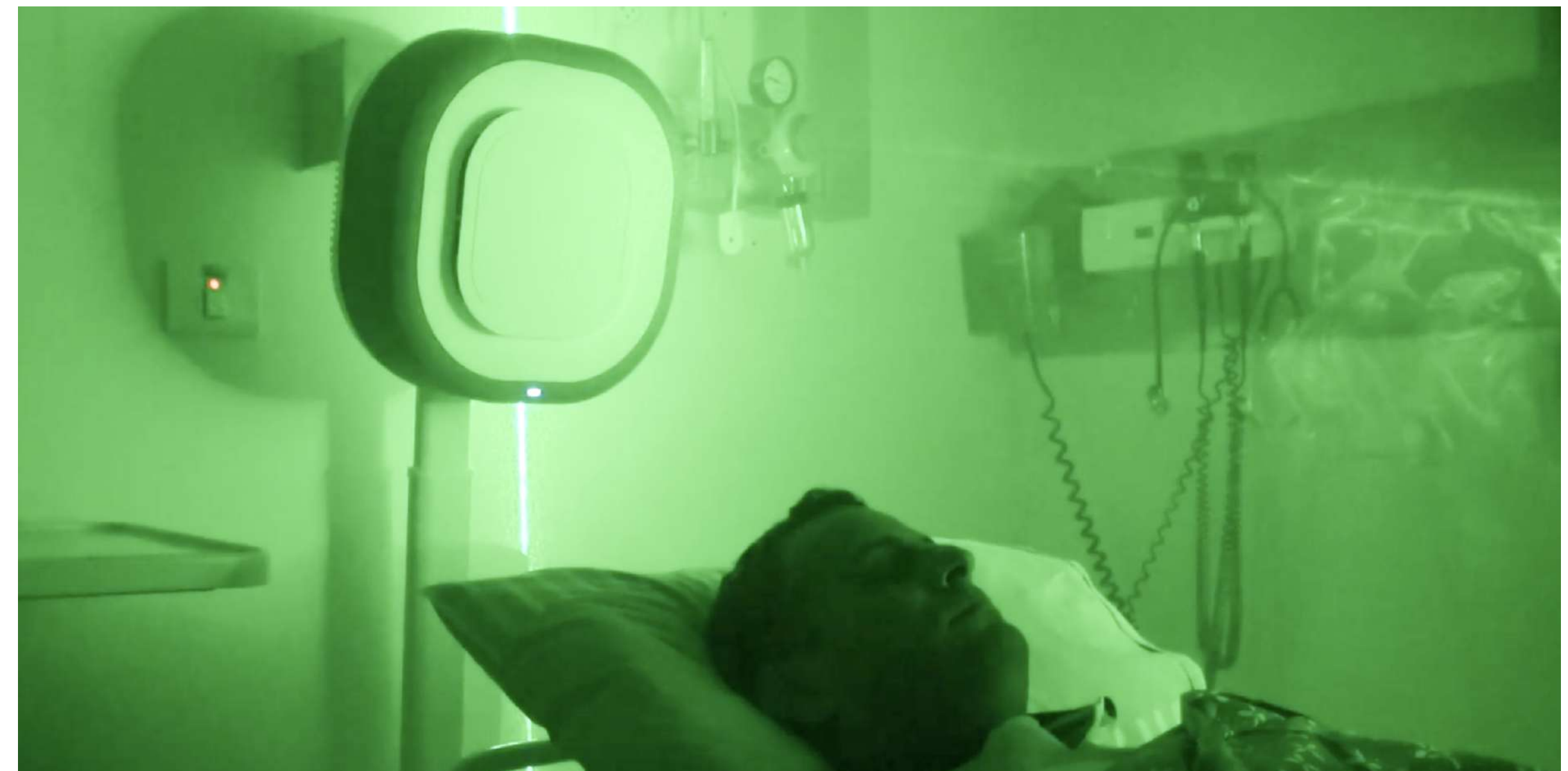
Using a laser light, smoke particles were illuminated in the room environment
