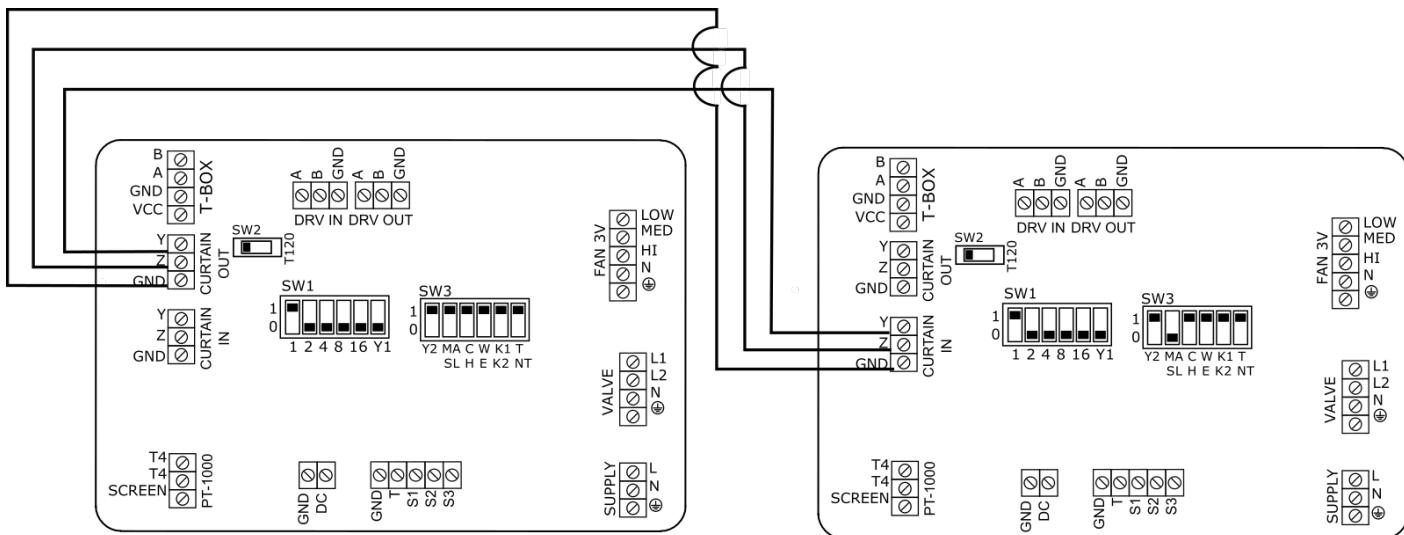
Electrical air curtain chaining provides control from 1 to 5 devices using one TS and DC.
