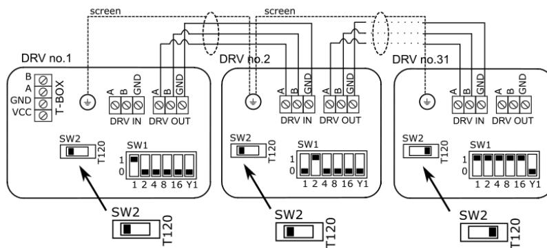
It is possible to connect up to 31 modules DRV and control them with one T-box controller.
