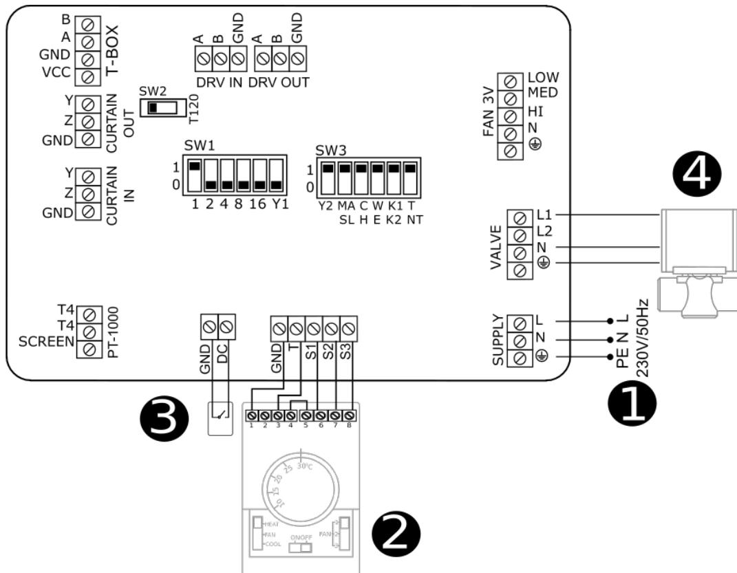
① Power supply 230 V/50 Hz (OMY min. 3x1 mm<sup>2</sup>) (Overcurrent B4)
