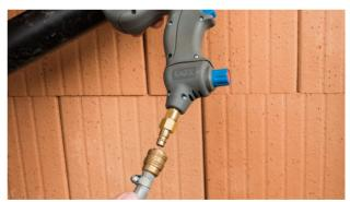
**6. Connect AEROFIXX** Connect the spray gun to the compressed air. Air requirement approx. 250 l/min. Set the pressure to 6 bar (87 psi) on the pressure reducer.
