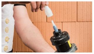
**5. Put on the air nozzle** Hand-tighten the air nozzle onto the spray head.
