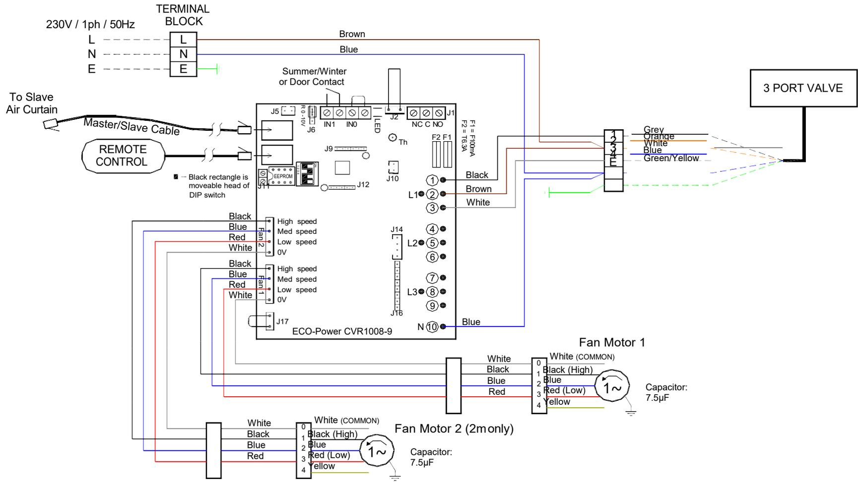
**APPENDIX 2D — WIRING DIAGRAM FRB1000W, FRB1500W and FRB2000W**
