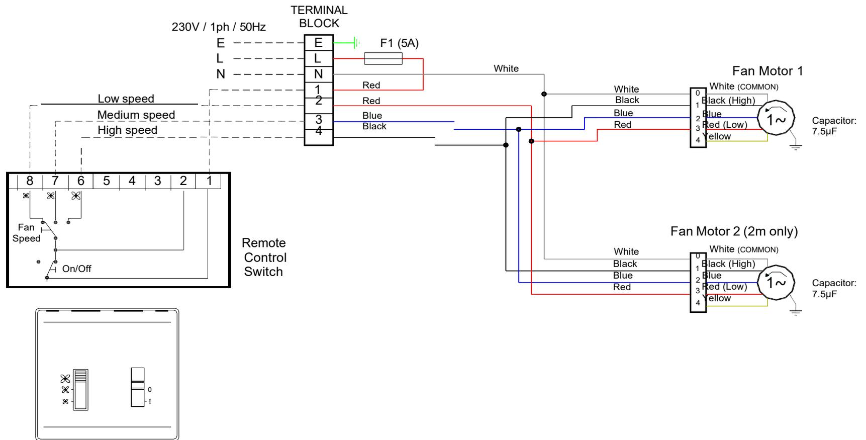
**APPENDIX 2E — WIRING DIAGRAM FRB1000A, FRB1500A and FRB2000A**
