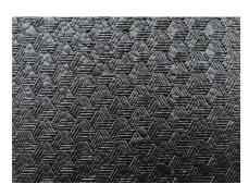
Body of the unit is made from black **EPP**. (expanded polypropylene). Water exchanger is controlled by thermostatic water valve.
