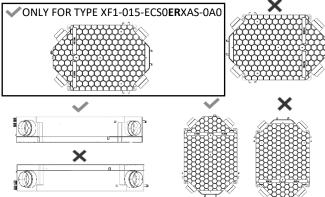
The Xflat unit must be installed and put into operation in accordance with the general and locally valid safety regulations, by a person with adequate education, experience and knowledge of the relevant regulations, standards and possible risks and possible dangers, or by a suitably trained service technician. Failure to follow the installation procedure may result in damage to the unit, malfunction, and possible injury to the user's health and property.
