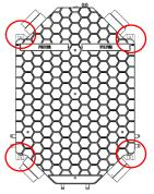
**b)** Choose the installation position taking into account the location of the condensate outlet. Align the anchor holes according to the dimensions on the unit, drill and mount the unit leveled using suitable screws. Do not tilt the unit.
