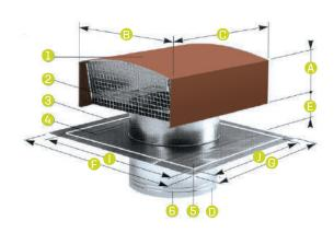
The metal sheath (3) that fits into the vent pipe is rigidly connected to both the support plate (4) that attaches to the roof frame and the malleable lead flashing (3)
