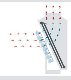
The evaporating energy of water is used to cool the incoming air.
