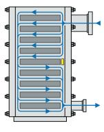
Vertical for Liquid-Liquid and Multipass Condensers and Evaporators
