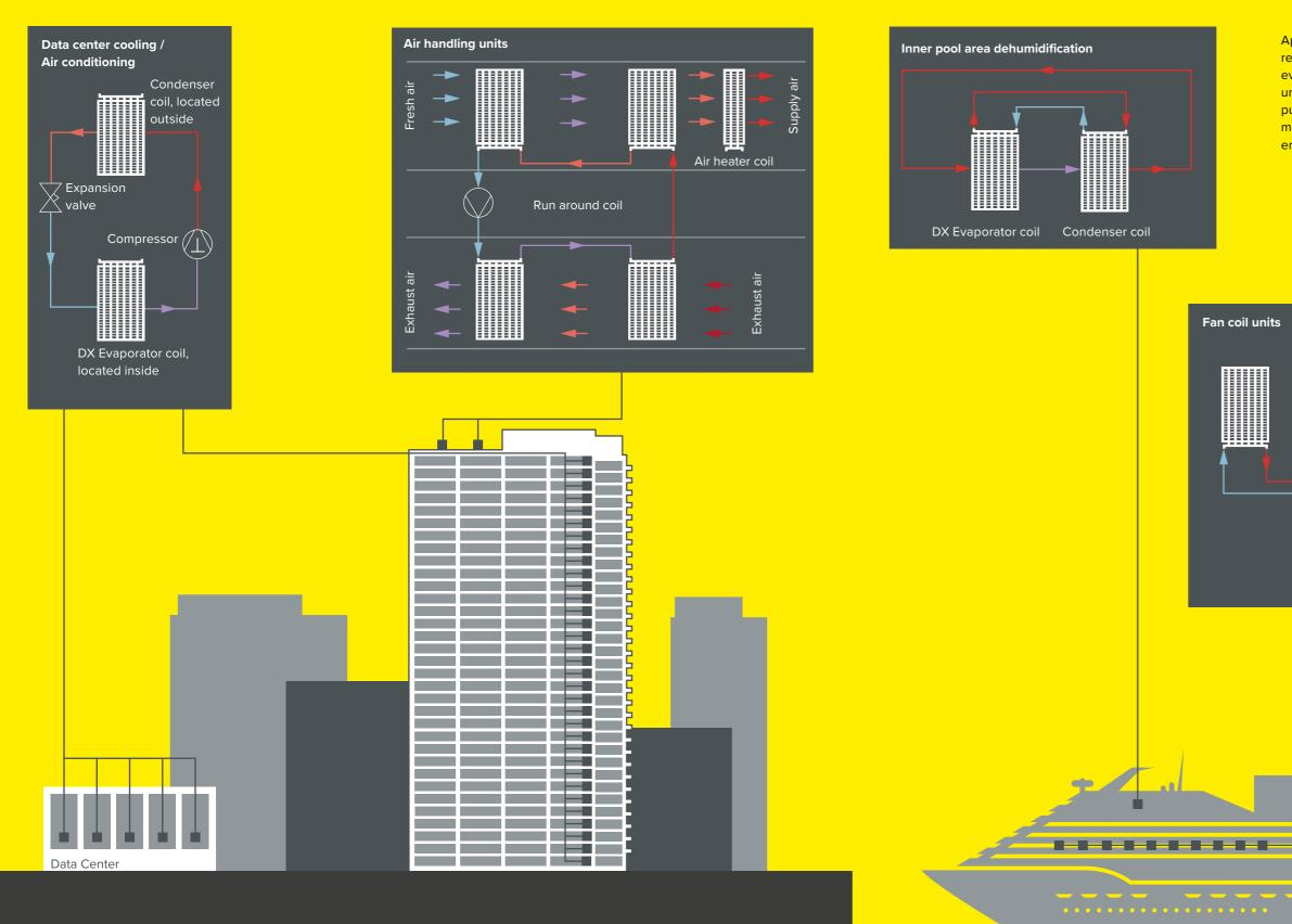
Applications for heat exchanger coils range from heat recovery and process heating to cooling, condensing and evaporating. They are suitable for air handling units, fan coil units, data center cooling, air drying systems, chillers, heat pumps, process water cooling, chilled beams, engine cooling, medical equipment, mining, gas turbine air pre-heating, energy recovery and much more.
