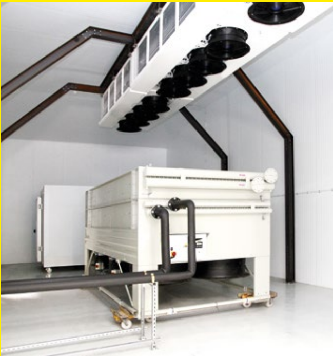
Unit under test in large calorimeter room
