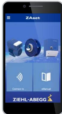
*A smartphone can be used to read out motor data wirelessly or via cable.*
